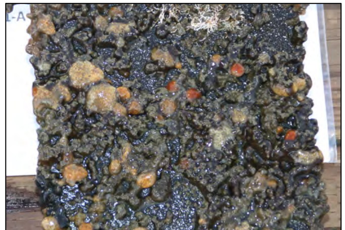
12 months’ fouling on copper-coated test-panel, San Diego Bay. Scott Parker
